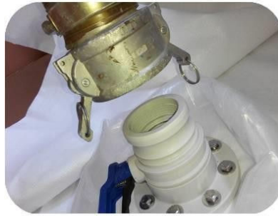
Clean the pipe& adaptor and connect the adaptor with the valve
