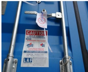
Close right door, put on the Caution Label on the LEFT Door, Make sure the container door is closed well before leave.
