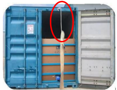
Use the string to hang the loading pipe and make sure it is vertical to the floor
