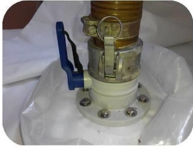
Connection of valve and pipe shall be upright, not being tilt. This will release the pressure to the bag.
