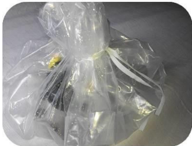
Cover the bonnet with string. (If have hose airvent, close the hose airvent cap)
